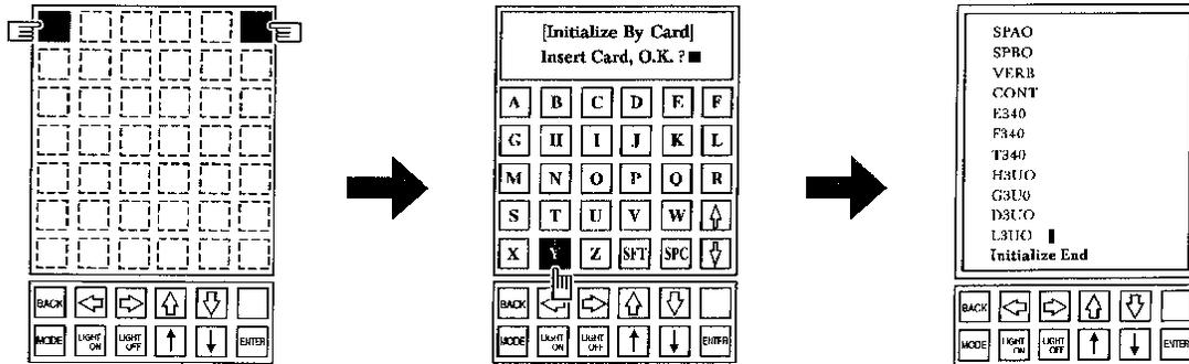
1. While holding down the upper left and right corner keys of the CONSULT touch panel, simultaneously press the power "ON" switch. While pushing the power "ON" switch, hold down both corner keys until the next screen appears.
