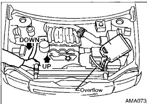
21. Pour more coolant into radiator while gently moving upper radiator hose up and down.
