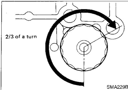
3. Screw in the oil filter until a slight resistance is felt, then tighten additionally more than 2/3 of a turn.
