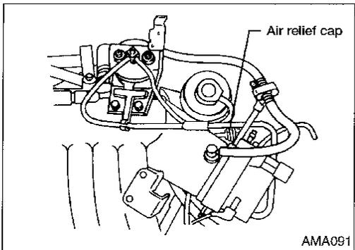
17. Remove heater pipe air relief cap.
