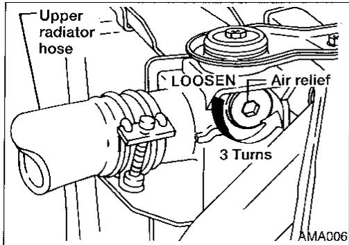
16. Loosen radiator air relief plug 3 turns.
