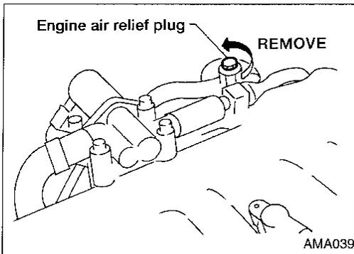
15. Remove engine air relief plug.
