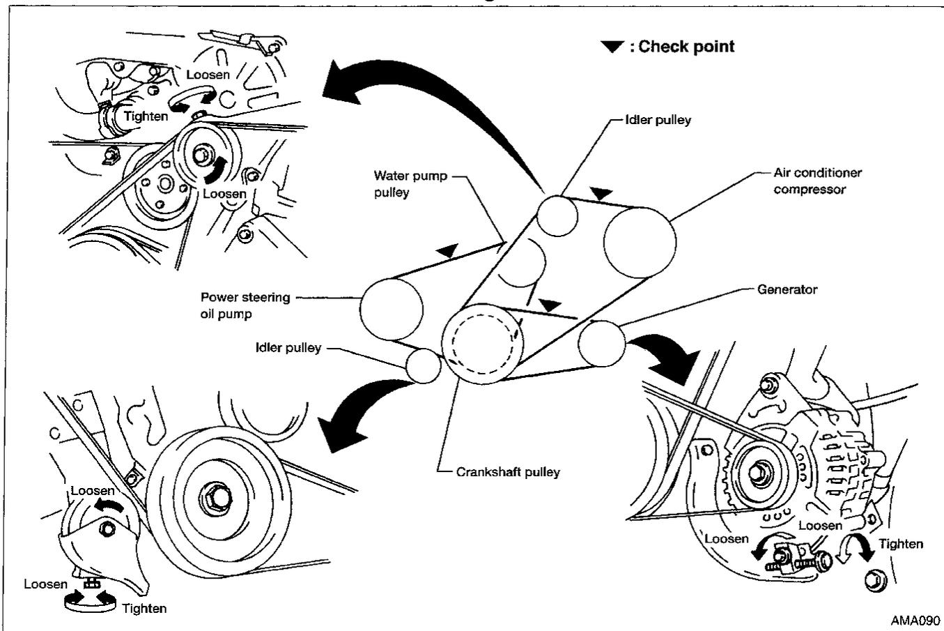
1. Inspect belts for cracks, fraying, wear and oil. If necessary, replace.
