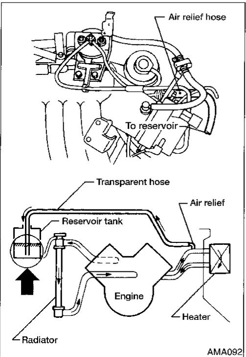
18. Install 1 meter (40") of 6 mm (0.24 in) I.D. heat resistant hose (clear if available, minimum temperature rating 105°C/ 220°F) to heater pipe air relief.
