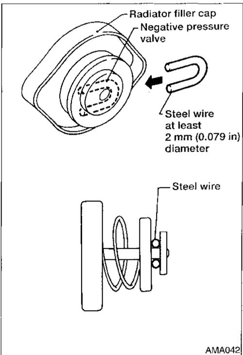
22. Install a wire under radiator filler cap negative pressure valve to allow flow of air and coolant regardless of pressure. **(Do not install cap.)**
