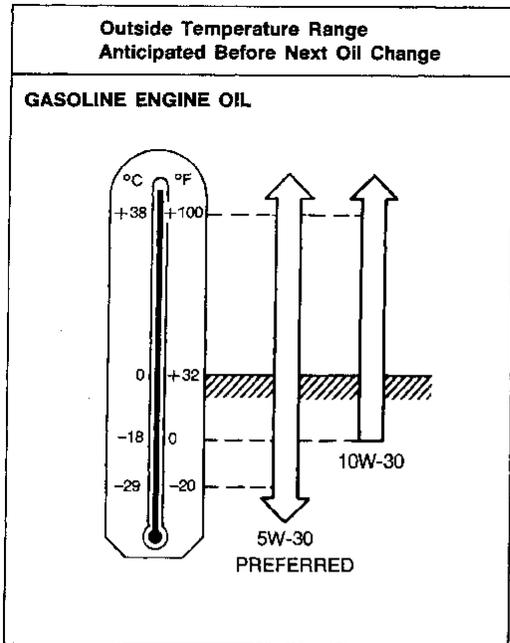
SAE 5W-30 viscosity oil is preferred for all temperatures. SAE 10W-30 viscosity may be used if the ambient temperature is above  $-18^{\circ}\text{C}$  ( $0^{\circ}\text{F}$ ).
