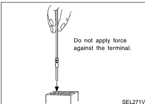
3. While holding the wire of the male terminal, try to insert the male terminal into the female terminal. **Do not force the male terminal into the female terminal with your hands.**
