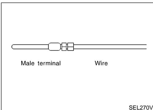
1. Assemble a male terminal and approx. 10 cm (3.9 in) of wire. **Use a male terminal which matches the female terminal.**
