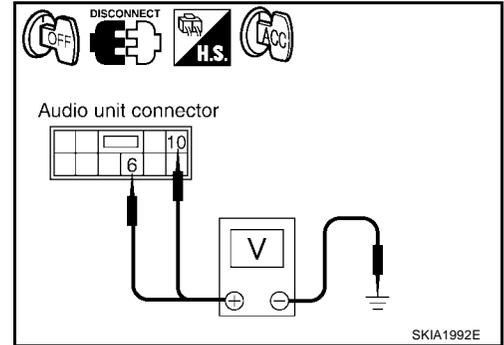
3. Check voltage between subwoofer (BOSE system) and ground.
