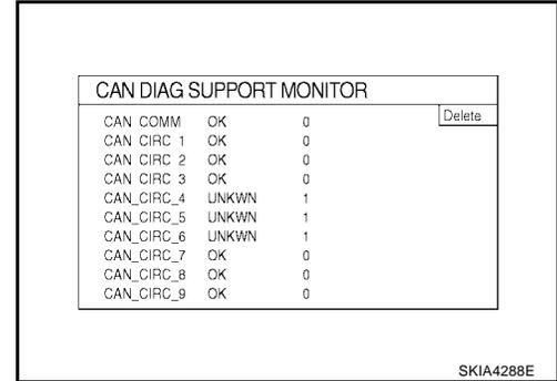
3. Record each item display description (OK/NG/UNKWN) displayed on the following CAN DIAG SUPPORT MONITOR Check Sheet.
