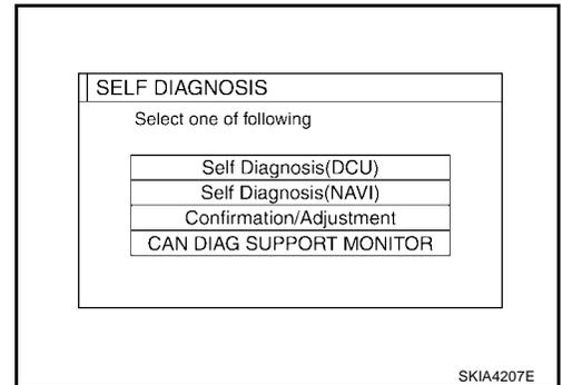
5. When "Confirmation/Adjustment" is selected on the initial trouble diagnosis screen, the operation will enter the CONFIRMATION/ADJUSTMENT mode. In this mode, check and adjustment of each item will become possible.
