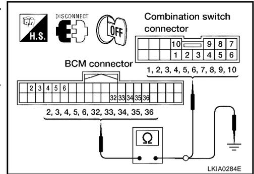
3. Check for continuity between each terminal of BCM harness connector in suspect malfunctioning system and ground.
