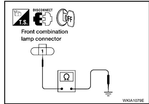
2. Check continuity between license lamp plate harness connector and ground.
