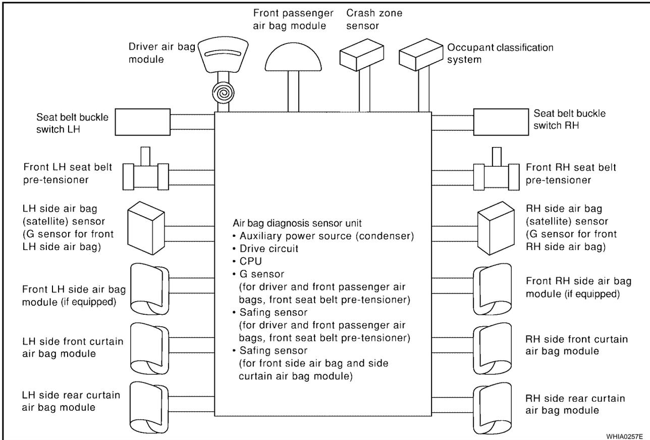
The air bag deploys if the air bag diagnosis sensor unit is activated while the ignition switch is in the ON or START position.
