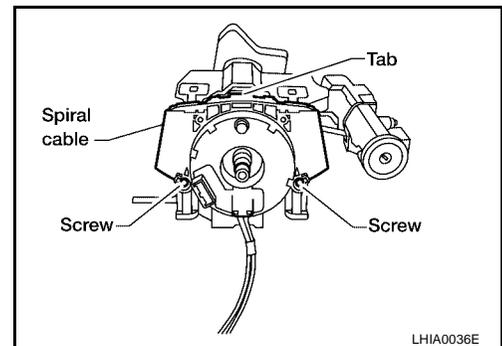
10. Remove the spiral cable connectors.
