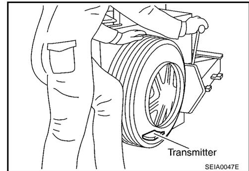
3. Turn tire so that valve hole is at bottom and bounce so that transmitter is near valve hole. Carefully lift tire onto turntable and position valve hole (and transmitter) 270 degrees from mounting/dismounting head.
