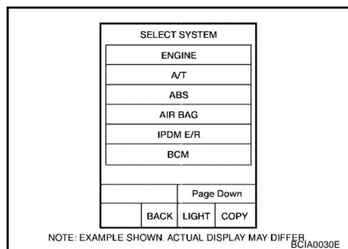
4. Touch appropriate item, "DATA MONITOR" or "ACTIVE TEST" on "SELECT DIAG MODE" screen.
