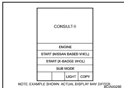
3. Touch "IPDM E/R" on "SELECT SYSTEM" screen. If "IPDM E/R" is not displayed, go to [GI-37, "CONSULT-II Data Link Connector \(DLC\) Circuit"](#).
