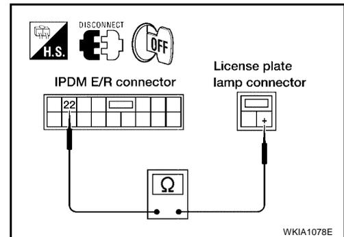
5. Check continuity between IPDM E/R harness connector and rear combination lamp harness connector.
