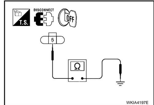
3. Check continuity between license lamp plate harness connector and ground.
