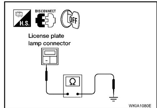
4. Check continuity between rear combination lamp harness connector and ground.
