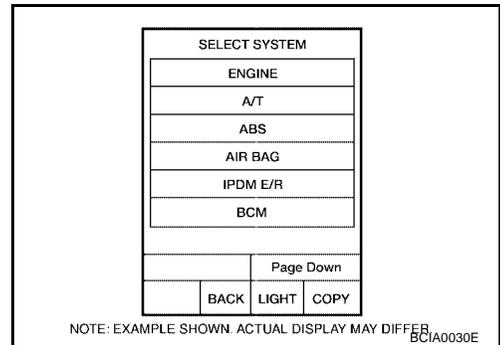
4. Select the desired part to be diagnosed on the "SELECT DIAG MODE" screen.
