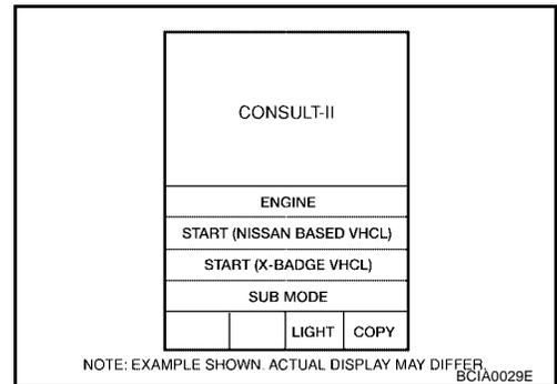
3. Touch "IPDM E/R" on "SELECT SYSTEM" screen. If "IPDM E/R" is not displayed, go to [GI-38, "CONSULT-II Data Link Connector \(DLC\) Circuit"](#).
