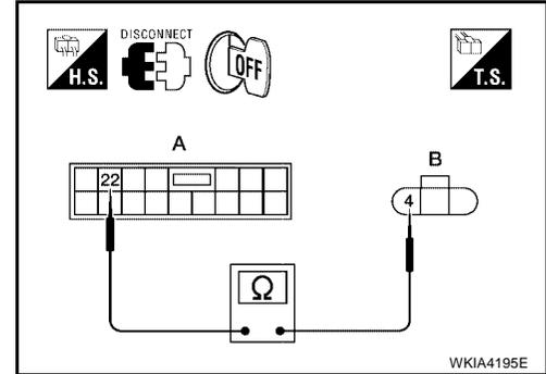
4. Check continuity between IPDM E/R harness connector and license plate lamp harness connector.
