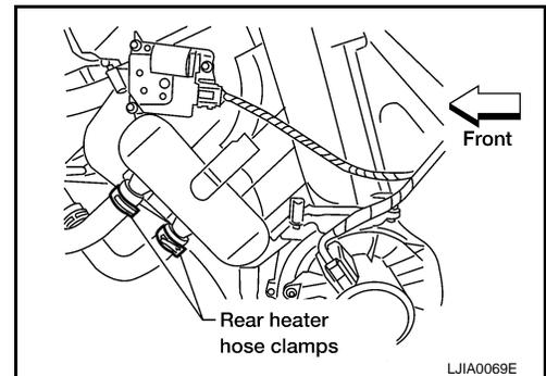
4. Remove the rear heater core bracket.
