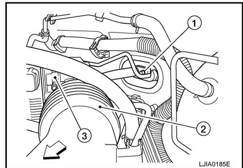
13. Use a suitable tool to pry the pipe support clip (1) from the threaded stud on the dash panel as shown.
