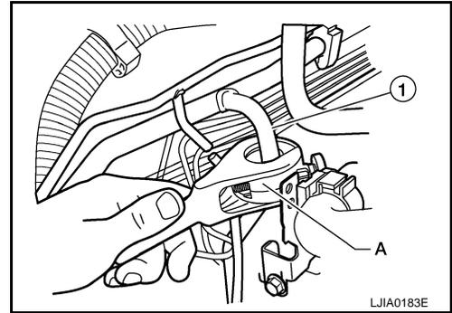
10. Disconnect the power brake booster vacuum hose from the intake manifold collector to allow removal of the cut A/C pipes.
