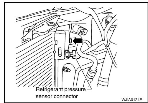
6. Carefully release retaining clips located on top driver side of condenser and rotate the condenser out of its mounts as shown.
