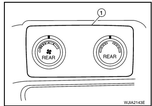
2. Disconnect the rear air control (rear) electrical connector and remove the rear air control (rear).
