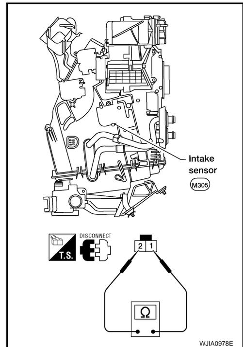
If NG, replace intake sensor. Refer to [ATC-132. "Removal and Installation"](#).
