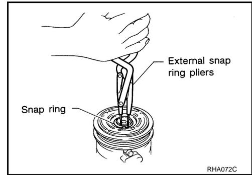
5. Remove the pulley assembly using Tool.
