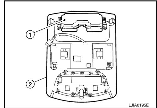
4. Remove the rear air control (front).
