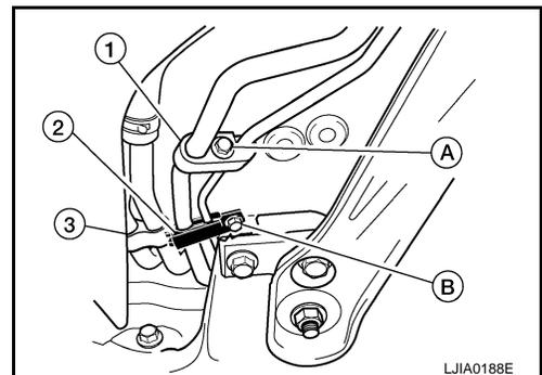
d. Attach the other pipe support clip to the dash panel threaded stud.
