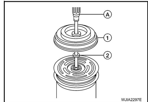
5. Install the center bolt using suitable tool (A).
