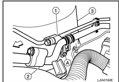
12. Disconnect the high/low pressure pipe connector bolt (1) from the front expansion valve as shown.
