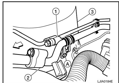
3. Complete the installation of the lower high/low pressure pipe.
