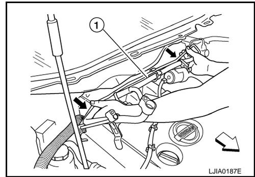
15. Remove the lower section of the high/low pressure pipe.
