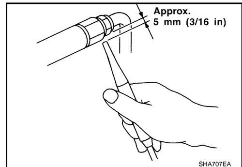
2. When checking for leaks, circle each fitting completely with the probe as shown.
