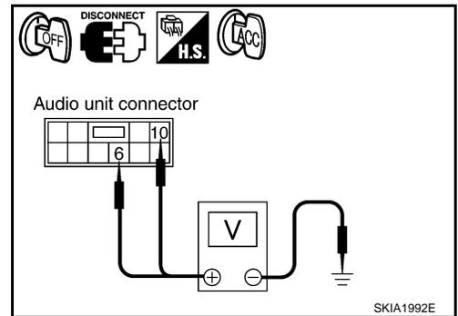
3. Check voltage between subwoofer (BOSE system) and ground.
