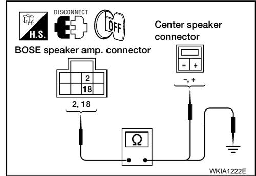
3. Check continuity between BOSE speaker amp. harness connector M113 terminals and ground.
