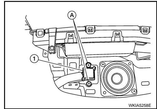
5. Disconnect GPS antenna connector and remove GPS antenna and feeder assembly out the top.
