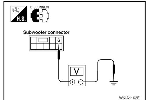
4. Check voltage between BOSE speaker amp. (with BOSE) and ground.
