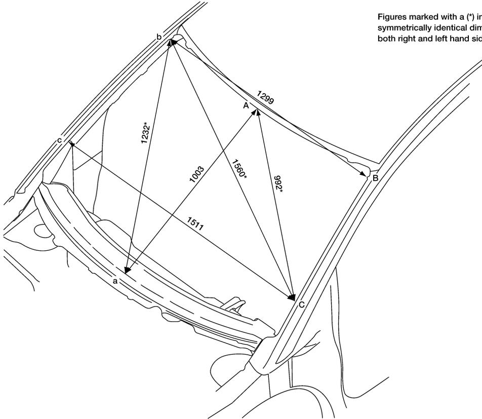
Figures marked with a (\*) indicate symmetrically identical dimensions on both right and left hand sides of vehicle.
