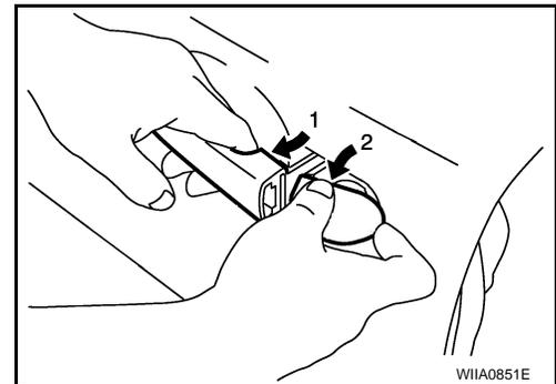
4. While pulling outside handle (1), slide toward rear of vehicle to remove (2).
