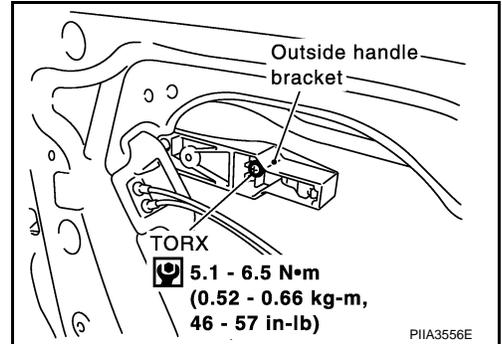
8. While pulling outside handle, slide toward rear of vehicle to remove outside handle and door lock assembly.
