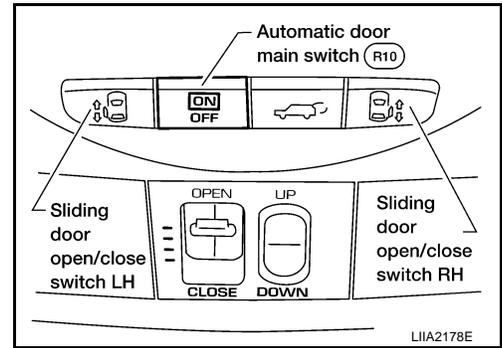
8. Press and HOLD the same overhead Sliding Door Open/Close Switch of the door being initialized again until the door completely opens and stops, then release the switch.
