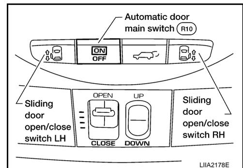
5. Press and HOLD the overhead Sliding Door Open/Close Switch again until the door completely opens and stops, then release the switch.
