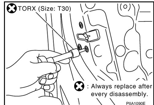
9. Remove the TORX bolt (T30) from the outside handle bracket.
