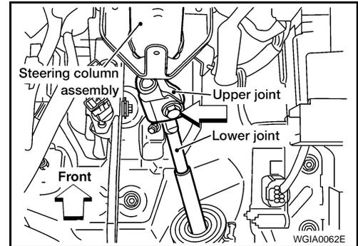
6. Remove nuts and bolt from steering member, remove steering column assembly from steering member.
