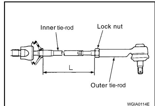
3. Measure rack stroke. Refer to [PS-25, "Steering Gear and Linkage"](#).
