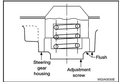
2. Loosen adjusting screw in 40° - 60° increments until rack sliding force is within specification. Refer to [PS-25. "Steering Gear and Linkage"](#).
