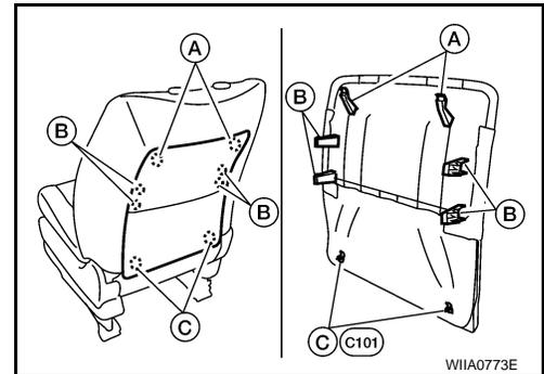
4. Remove the bolts (2 for each side) and seatback assembly.
