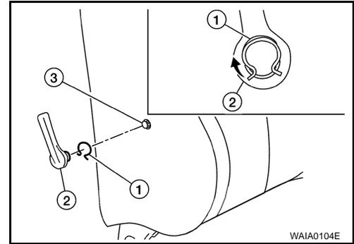
9. Disconnect the seatback heater harness. Remove the seatback trim and pad assembly. Remove the hog ring to separate the seatback trim from the pad and the heater unit.
