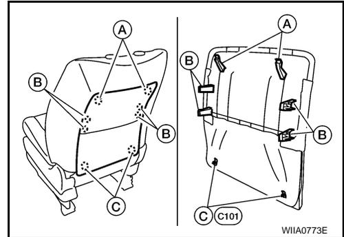
4. Remove the seatback board from the back of the seatback.
