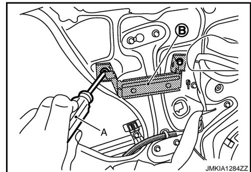
4. Remove the sealing screen by using a cutter tool.
