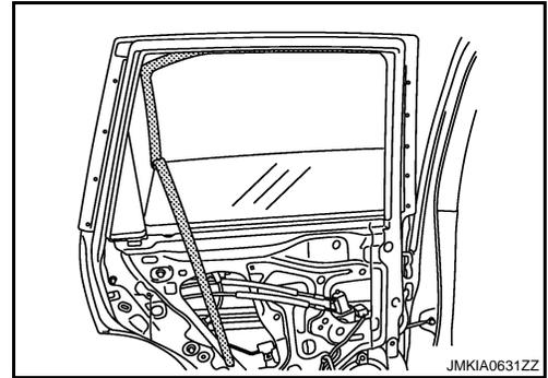
6. Remove the corner piece assembly fixing screws, then remove the corner piece assembly.
