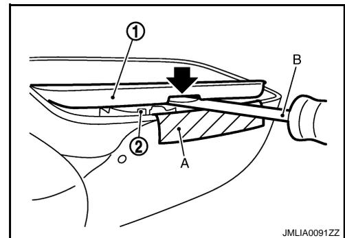
4. Insert a small slotted screwdriver at RH/LH side between glass mirror and actuator, and push up pawls to remove glass mirror RH/LH side.
