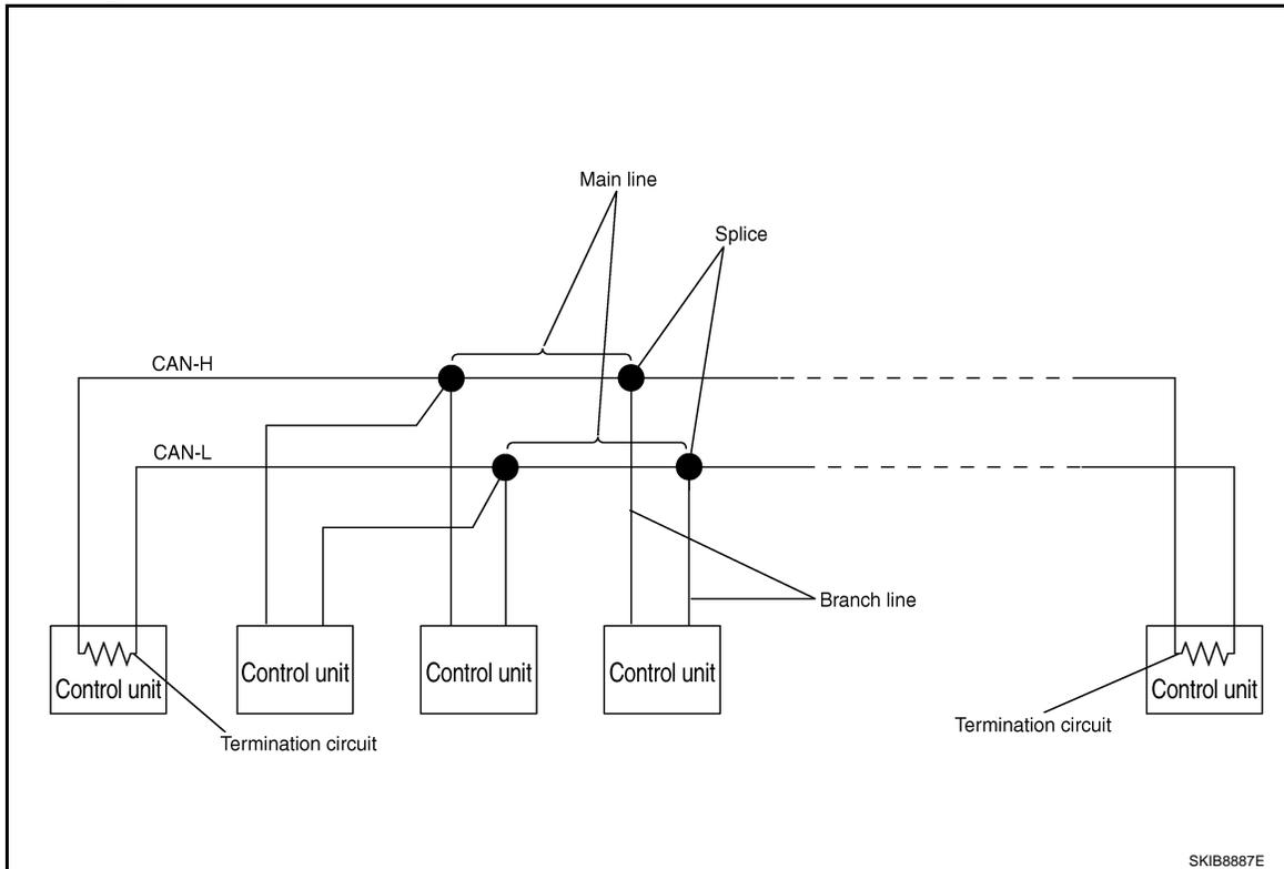
Each control unit passes an electric current to the termination circuits when transmitting CAN communication signal. The termination circuits produce an electrical potential difference between CAN-H and CAN-L. CAN communication system transmits and receives CAN communication signals by the potential difference.
