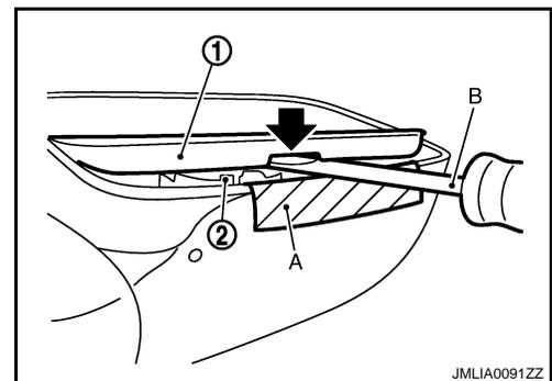
4. Insert a small flat-bladed screwdriver at LH/RH side between glass mirror and actuator, and push up pawls to remove glass mirror LH/RH side.
