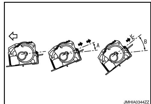
3. Replace the seat belt assembly if it does not operate normally.
