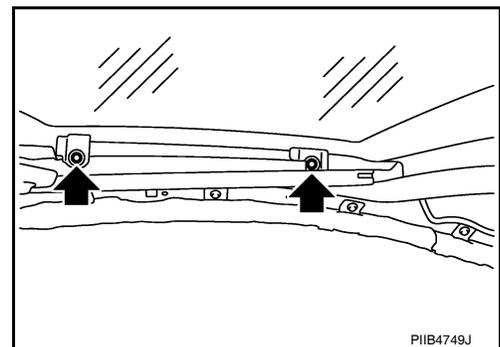
5. Tilt glass lid up and down several times to check that it moves smoothly, and retains the adjustment.
