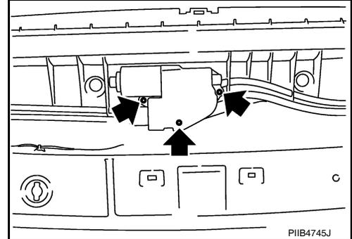
6. Remove the side and front sunroof unit assembly nuts.
