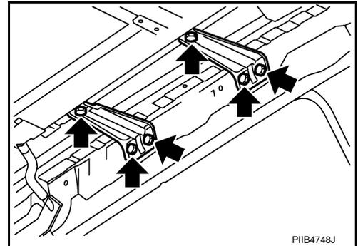
7. Connect the sunroof motor assembly connector and install the screws.
