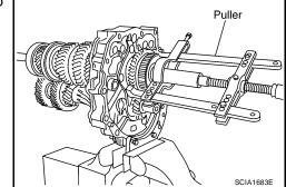
6. Remove reverse coupling sleeve according to the following. PCIB1236E
