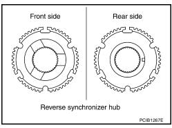
Install spread springs to shifting inserts to reverse synchronizer b. hub.
