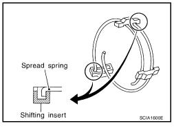
• Be careful with the shape of reverse shifting insert to avoid misassembly.
