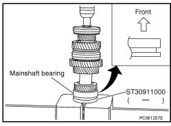
10. Press in reverse main gear bushing using Tool.
