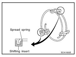
• Be careful with the shape of 1st-2nd, 3rd-4th and 5th-6th shifting insert to avoid misassembly.
