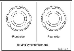
b. Install spread springs and shifting inserts to 1st-2nd synchronizer hub.
