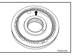
d. Press in reverse synchronizer hub assembly, reverse baulk ring, reverse main gear and reverse main needle bearing using Tools.
