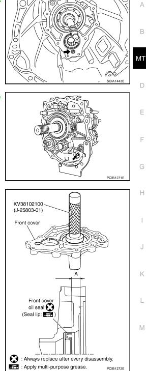
10. Install front cover oil seal to front cover using Tool.
