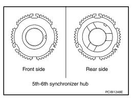
b. Install shifting inserts and spread springs to 5th-6th synchronizer hub.
