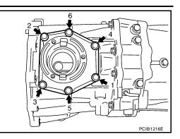
25. Install gasket to drain plug, and then install it to transmission case. Tighten drain plug to the specified torque. Refer to <u>MT-22</u>, <u>"Case Components"</u>.
