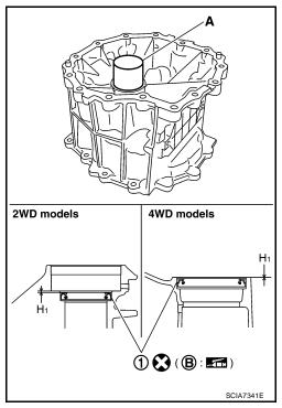
16. Install dust seal (1) to rear extension using Tool A (for 2WD models).
