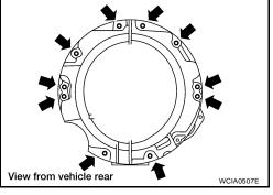
Improper alignment caused by missing dowels may cause vibration, oil leaks or breakage of drive train components.
