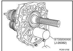
21. Install snap ring to mainshaft bearing. CAUTION: Do not reuse snap ring.
