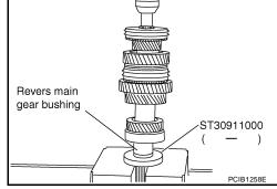
11. Press in 3rd gear bushing using Tool.
