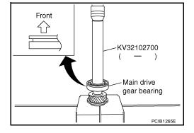
b. Select and install a snap ring to main drive gear bearing so that the end play comes within the standard value. Refer to  $\underline{\text{MT-70}}, \underline{\text{"Snap Rings"}}$ .
