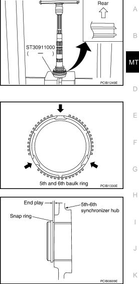
2. Select and install a snap ring so that the end play comes within the standard value. Refer to <u>MT-70, "Snap Rings"</u>.
