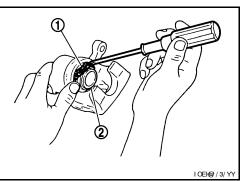
Install the piston (1) into the cylinder body and insert the piston boot (2) side lip into the piston groove as shown.
