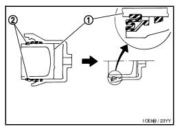
Apply rubber grease to the sliding pin boots, then install the new upper sliding pin, lower sliding pin, and sliding pin boots on the torque member.
