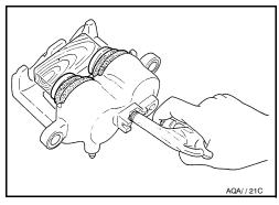
Remove the piston boots from the pistons. 4. CAUTION: Do not reuse piston boot.
