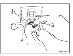
3. Apply rubber grease to the new piston boot (1). Cover the piston end (2) with the piston boot (1), and then install the cylinder side lip on the piston boot (1) securely into the groove on the cylinder body.
