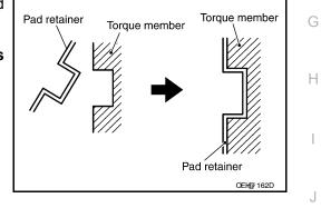
3. Attach pad retainer to torgue member, then install brake pad and shim assemblies. CAUTION:
