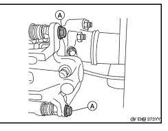
Connect the brake hose to the caliper body, using a new copper washer. Tighten the hose connection (A) to the specified torque. Refer to <u>BR-12, "Hydraulic Circuit"</u>. CAUTION:
