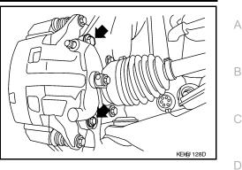
5. Install brake hose by aligning with the protrusion on caliper body, then install new copper washers and union bolt. Tighten union bolt to specified torque. Refer to BR-33, "Exploded View of Brake Caliper". **CAUTION:**
