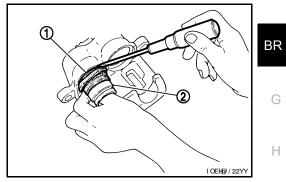
Install the pistons (1) into the cylinder body and insert the piston boots (2) side lip into the piston groove as shown.
