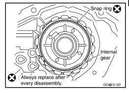
Install the planetary carrier assembly and sun gear assembly to the front case using Tool.
