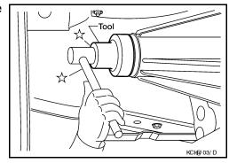
2. Apply petroleum jelly to the circumference of the new dust cover. Position the new dust cover as shown.
