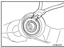
Remove differential side shaft assembly out of gear carrier using suitable tool.
