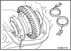
13. Remove side bearing adjusters from axle housing.
