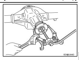
Remove front oil seal using Tool.
