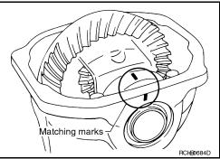
To determine side bearing preload torque, measure the pulling force of the differential assembly at the drive gear bolt using Tool.
