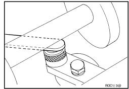
10. Write down the exact measurement (the value of feeler gauge).
