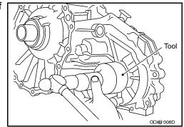
37. Align the matching mark on the front drive shaft with the mark on the companion flange, then install the companion flange.
