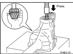
6. Remove the drive pinion rear bearing inner race and drive pinion height adjusting washer using Tool.
