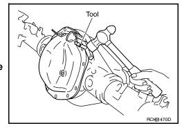
3. For proper reinstallation, paint matching marks on one side of side bearing cap.
