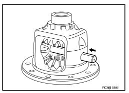
Drive a new lock pin into the pinion mate shaft until it is flush with the differential case using suitable tool. CAUTION:
