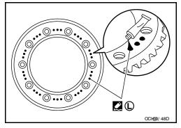
2. Align the matching mark of differential case assembly with the mark of drive gear, then install drive gear.
