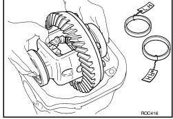
Insert the left and right original side bearing adjusting washers in place between side bearings and gear carrier using Tool.
