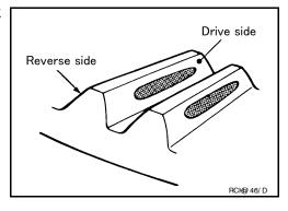
• If the tooth contact is improperly adjusted, adjust the drive pinion height (dimension X).
