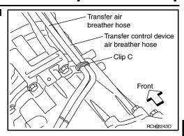
Install transfer control device air breather hose and transfer air breather hose on clip D with the paint mark facing upward.
