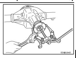
Remove front oil seal using Tool.
