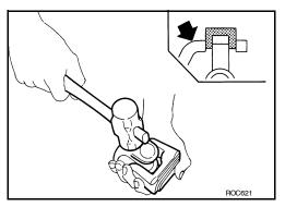
4. Make sure that the journal moves smoothly and is below the propeller joint flex effort specification. Refer to <u>DLN-142</u>, "General Specification".
