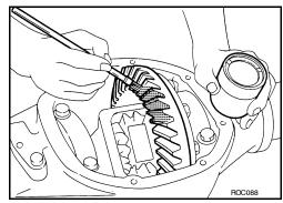
Rotate the drive gear back and forth several times. Then check for correct drive pinion to drive gear tooth contact as shown. CAUTION:
