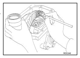
Rotate the drive gear back and forth several times. Then check for correct drive pinion to drive gear tooth contact as shown. CAUTION:
