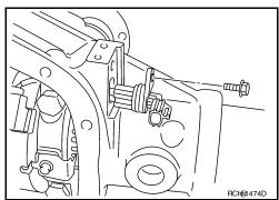
4. For proper reinstallation, paint matching mark on one side of side bearing cap.
