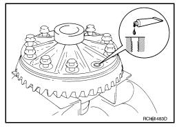
Install new drive gear bolts, and then tighten to the specified torque. Refer to <u>DLN-223</u>, "<u>Disassembly and Assembly</u>".
