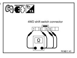
4. If the inspection results are abnormal replace the 4WD shift switch.
