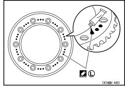
9. Align the matching mark of differential case with the mark of drive gear, then install drive gear.
