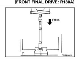
5. Apply multi-purpose grease to the lips and differential gear oil to the circumference of the new side oil seal. Then drive the new side oil seal in evenly until it becomes flush with the gear carrier using Tools.
