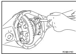
11. Loosen the side bearing adjusters using Tool.
