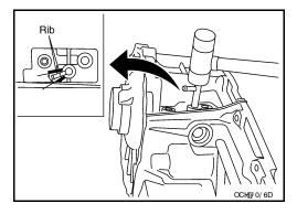
2. Install the baffle plate to the front case. Tighten the bolt to the specified torque. Refer to <u>DLN-102</u>, "<u>Disassembly and Assembly</u>".
