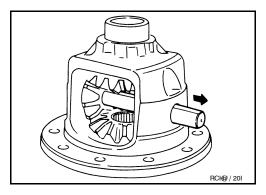
12. Turn the pinion mate gear, then remove the pinion mate gear, pinion mate thrust washer, side gear and side gear thrust washer from differential case.
