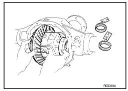
6. Remove side bearing inner race using Tools.
