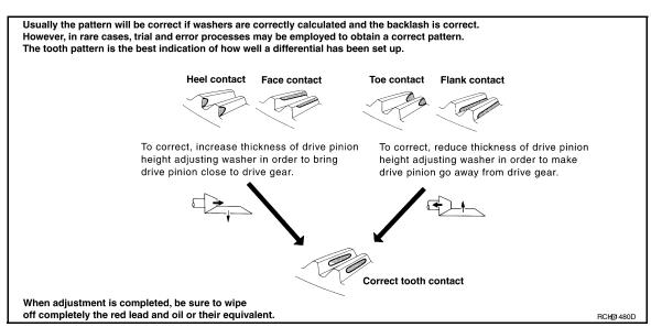
4. If outside the standard, adjust drive pinion height adjusting washer and backlash. Refer to <u>DLN-295</u>, "<u>Disassembly and Assembly</u>" and <u>DLN-310</u>, "<u>Inspection and Adjustment</u>".
