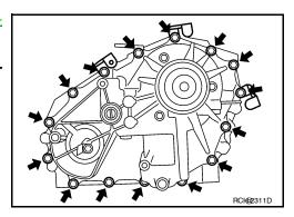
: Apply Genuine Anaerobic Liquid Gasket.
