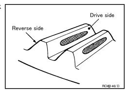
3. If the tooth contact is improperly adjusted, follow the procedure below to adjust the pinion height (dimension X).
