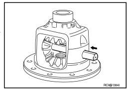
6. Drive a new lock pin into the pinion mate shaft until it is flush with the differential case using suitable tool.
