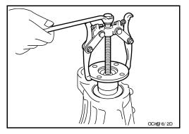
Press the drive pinion assembly (with rear inner bearing race and collapsible spacer) out of the gear carrier.CAUTION:
