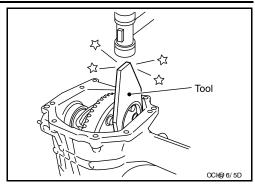
14. Install the side bearing caps with the matching marks aligned and tighten the side bearing cap bolts to the specified torque. Refer to <u>DLN-158</u>, "<u>Disassembly and Assembly</u>".
