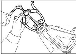
5. Remove the front oil seal using suitable tool.
