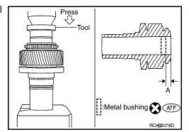
2. Apply ATF to the new needle bearing, then install the new needle bearing until it becomes "Dimension B" using Tool.
