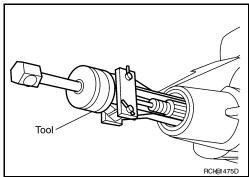
7. Remove drive pinion assembly (with rear inner bearing race and collapsible spacer) out of gear carrier.
