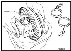
13. Insert the selected left and right side bearing adjusting washers in place between the side bearings and gear carrier using Tool.
