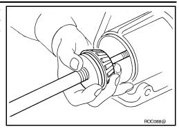
Turn the assembly several times to seat the drive pinion bearings.
