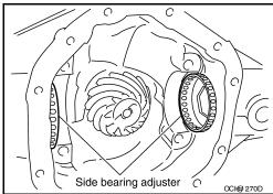
14. Apply gear oil to side bearings. Install differential case assembly with side bearing outer races into gear carrier.
