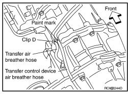
Install transfer air breather hose into the breather tube (transfer, metal connector) until the hose end reaches the base of the tube. Set transfer air breather hose with paint mark facing upward.
