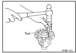
14. Remove pinion mate shaft.
