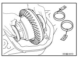
9. Remove side bearing inner races using Tool.
