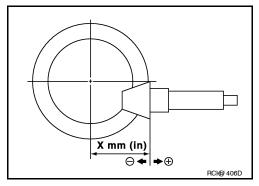
If the tooth contact is near the face (face contact), or near the heel (heel contact), use a thicker drive pinion height adjusting washers to move the drive pinion closer to the drive gear.
