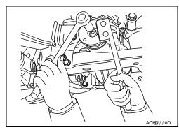
Remove the companion flange using suitable tool.
