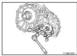
7. Remove the front oil seal from the front case using Tool.
