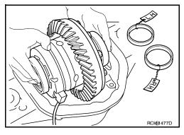
13. Connect differential lock solenoid harness and sensor connector. Then install it to gear carrier, tighten to the specified torque. Refer to <u>DLN-295</u>, "<u>Disassembly and Assembly</u>".
