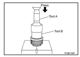
Install the new snap ring to the sun gear assembly using suitable tool.
