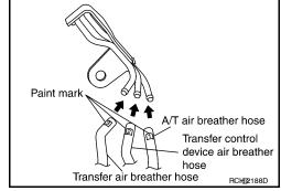
Install transfer control device air breather hose and transfer air breather hose on clip A and clip B with the paint mark facing upward.
