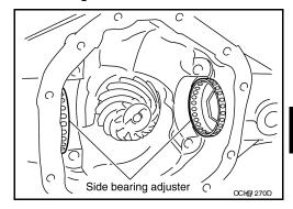
4. Apply gear oil to side bearings. Install differential case assembly with side bearing outer races into axle housing.
