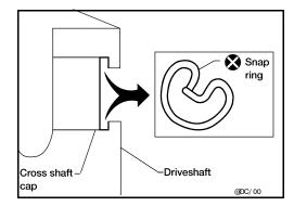
Push out and remove the journal bearings by lightly tapping the flange yoke with a hammer, taking care not to damage the journal or flange yoke hole.
