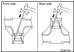
11. Remove drive pinion rear bearing inner race and drive pinion height adjusting washer using Tool.
