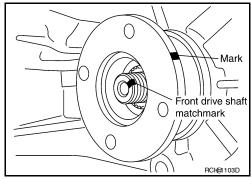
3. Install the new self-lock nut and tighten to the specified torque, using Tool. Refer to <a href="DLN-102">DLN-102</a>, "Disassembly and Assembly".
