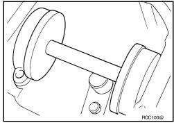
9. Select the correct standard drive pinion height adjusting washer thickness. Select by using a standard gauge of 3 mm (0.12 in) and your J-34309-101 feeler gauge. Measure the distance between the J-34309-10 drive pinion height adapter, including the standard gauge and the arbor.
