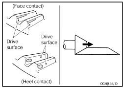
If the tooth contact is near the flank (flank contact), or near the toe (toe contact), use a thinner drive pinion height adjusting washers to move the drive pinion farther from the drive gear.
