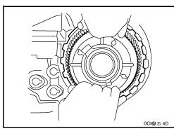
34. Remove the snap ring from the front case.
