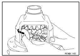
4. Install the pinion mate shaft and align the lock pin hole on the pinion mate shaft with the lock pin hole on the differential case.
