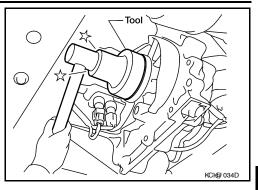
2. Align the matching mark of the front drive shaft with the matching mark of the companion flange, then install the companion flange.
