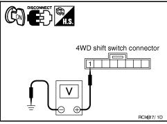
Transfer control unit connector 4WD shift switch connector RCH@2255D
