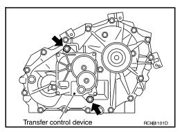
41. Install the drain plug and filler plug with new gaskets to the rear case. Tighten to the specified torque. Refer to <a href="DLN-102">DLN-102</a>, "Disassembly and Assembly". CAUTION:
