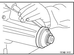
11. Remove the rear oil seal from the rear case using Tool.
