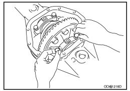
16. Tighten each side bearing adjusters using Tool.
