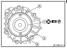
33. Install the new dust cover to the rear case using Tool.
