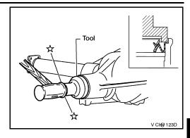
3. Align the matching mark of drive pinion with the matching mark A of companion flange, then install the companion flange.
