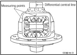
Using feeler gauges, measure the clearance between the side gear back and differential case at three different points, while rotating the side gear. Average the three readings to calculate the clearance. (Measure the clearance of the other side as well.)
