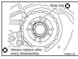
35. Remove the input bearing from the front case using Tool.
