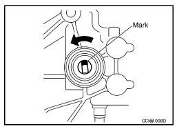
b. Align the transfer control device shaft cutout with the mark on the control shift rod, and install.
