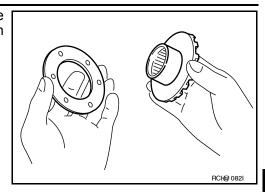
2. Install the side gears and side gear thrust washers into the differential case.
