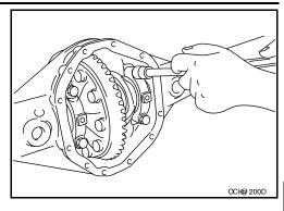
6. Remove side bearing adjusters using Tool.
