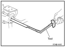
7. Place the J-34309-11 drive pinion height adapter onto the gauge plate and tighten it by hand.
