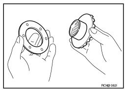
Install the side gears and side gear thrust washers into the differential case.
