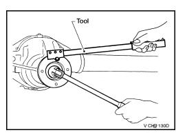
Remove the companion flange using suitable tool.
