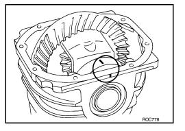
15. Check and adjust the drive gear runout, tooth contact, drive gear to drive pinion backlash, and total preload torque. Refer to "disassembly". Recheck above items. Α
