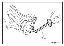
• If the measured value is out of the specification, check and adjust each part. Adjust the drive pinion bearing preload torque first, then adjust the side bearing preload torque.
