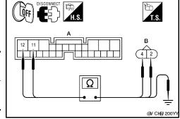
Check continuity between differential lock control unit harness connector M70 (A) terminals 11, 12 and ground.
