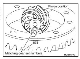
• The mounting distance from the center line of drive gear to the back face of drive pinion for the Model 226 final drive assembly is 109.5 mm (4.312 in).
