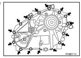
15. Separate the front case from the rear case. Then remove the rear case by prying it up using suitable tool.
