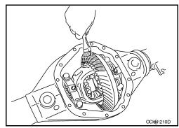
3. Hold companion flange steady by hand and rotate drive gear in both directions.
