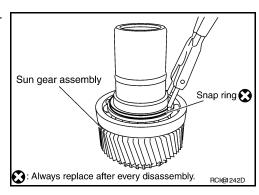
4. Remove the carrier bearing from the sun gear using Tools.
