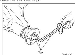
If the total preload torque is greater than specification
