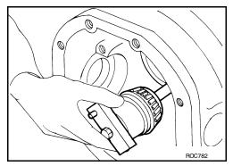
4. Assemble the drive pinion front bearing inner race and the J-34309-2 gauge anvil. Assemble them together with the J-34309-1 gauge screw in the gear carrier. Make sure that the drive pinion height gauge plate, J-34309-16, will turn a full 360°. Tighten the two sections together by hand.
