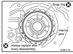
33. Remove the internal gear from the front case.
