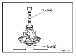
13. Install side bearing adjusters into gear carrier.
