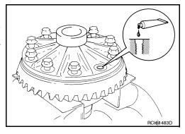
Tighten the drive gear bolts to the specified torque. Refer to <u>DLN-190</u>. "<u>Disassembly and Assembly</u>". After tightening the drive gear bolts to the specified torque, tighten an additional 31° to 36° using Tool.
