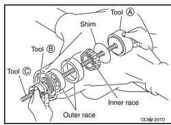
4. Turn the assembly several times to seat drive pinion bearings.
