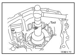
4. Install the new snap ring to the front case.
