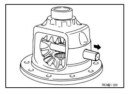
15. Turn the pinion mate gear, then remove the pinion mate gear, pinion mate thrust washer, side gear and side gear thrust washer from differential case.
