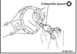
10. Install the companion flange onto the drive pinion while aligning the matching marks. Then tap the companion flange using suitable tool.
