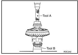
11. Install the differential case assembly with the side bearing outer races into gear carrier.
