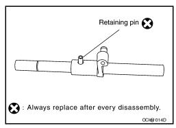
6. Install the drum cam to the control shift rod, and then secure it with the new retaining pin.
