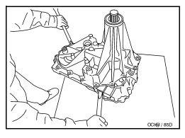
17. Remove the snap ring from the mainshaft using suitable tool.
