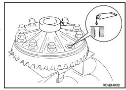
9. Tighten the new drive gear bolts to the specified torque. Refer to <u>DLN-158</u>, "<u>Disassembly and Assembly</u>". After tightening the new drive gear bolts to the specified torque, tighten an additional 34° to 39° using Tool.
