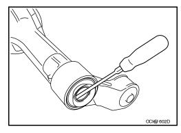
Remove snap ring (hole side) using suitable tool.
