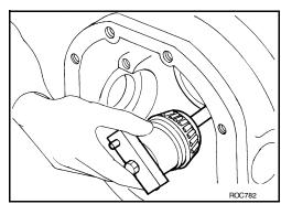
Assemble the drive pinion front bearing inner race and the J-34309-2 gauge anvil. Assemble them together with the J-34309-1 gauge screw in the gear carrier. Make sure that the drive pinion height gauge plate, J-34309-16, will turn a full 360°. Tighten the two sections together by hand.
