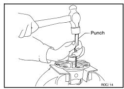
12. Remove the pinion mate shaft.
