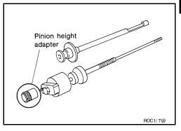
8. Position the side bearing discs, Tool, and arbor firmly into the side bearing bores. Install the side bearing caps and tighten the side bearing cap bolts to the specified torque. Refer to "COM-PONENTS".
