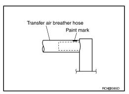
Install transfer control device air breather hose into transfer control device (case connector) until the hose end reaches the base of the tube. Set transfer control device air breather hose with paint mark facing forward.
