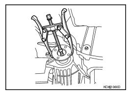
7. Remove the front oil seal using Tool.
