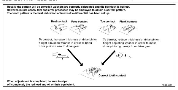
4. If outside the standard, adjust drive pinion height adjusting washer and backlash. Refer to <a href="DLN-223">DLN-223</a>, "Disassembly and Assembly" and <a href="DLN-239">DLN-239</a>, "Inspection and Adjustment".
