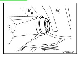
Remove the rear oil seal from the rear case using Tool. CAUTION:
