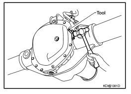
8. For installation, apply a paint matching mark on one side of side bearing cap.
