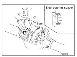
14. Install the side bearing caps with the matching marks aligned and tighten the side bearing cap bolts to the specified torque. Refer to <u>DLN-190</u>, "<u>Disassembly and Assembly</u>".
