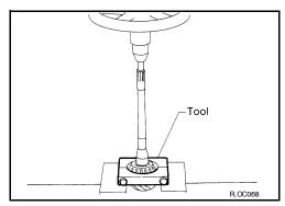
10. Tap drive pinion front and rear bearing outer races uniformly with a brass bar or equivalent to remove.
