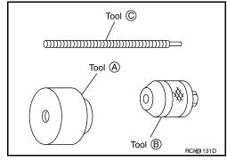
3. Install drive pinion bearing inner race and drive pinion height adjusting washer to gear carrier using Tool as shown.
