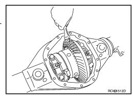
Hold companion flange steady by hand and rotate drive gear in both directions.
