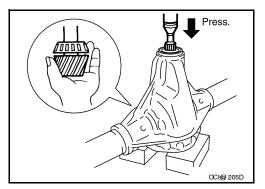
9. Tap drive pinion front bearing outer race uniformly with a brass bar or equivalent to remove.
