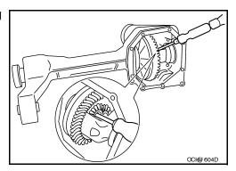
7. Press differential side shaft out of differential side shaft bearing. CAUTION:
