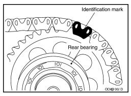
15. Install the drive chain together with the front drive shaft and sprocket to the front case.
