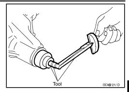
6. Tighten side bearing caps to the specified torque installing Tools as shown.
