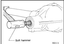
Remove drive pinion rear bearing inner race and drive pinion height adjusting washer using Tool.
