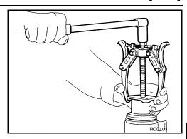
5. Remove drive pinion assembly from gear carrier using suitable tool.
