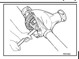
Keep side bearing outer races together with inner races. Do not mix them up. Also, keep side bearing adjusting washers together with bearings.
