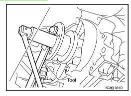
4. Put a matching mark on top of the front drive shaft in line with the mark on the companion flange.
