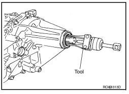
12. Remove the input oil seal from the front case using suitable tool. CAUTION:
