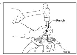
11. Remove pinion mate shaft.
