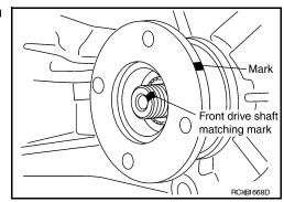
38. Install the new companion flange self-lock nut. Tighten to the specified torque using Tool. Refer to <a href="DLN-102">DLN-102</a>, "Disassembly and Assembly".
