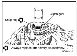
Install the new snap ring to the mainshaft using suitable tool.CAUTION:
