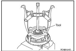
10. For proper reinstallation, paint matching mark on differential case and drive gear.
