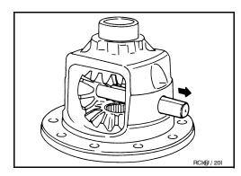
13. Turn the pinion mate gear, then remove the pinion mate gear, pinion mate thrust washer, side gear and side gear thrust washer from the differential case.
