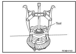
14. Remove side bearing inner race using Tool.
