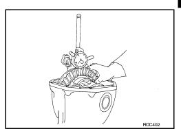
Do not change the total thickness of side bearing adjusting washers as it will change the side bearing preload torque.
