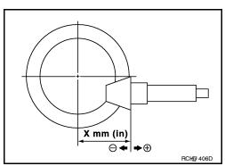
If the tooth contact is near the face (face contact), or near the heel (heel contact), use a thicker drive pinion height adjusting washer to move drive pinion closer to the drive gear.
