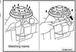
11. Remove the lock pin of the pinion mate shaft from the drive gear side using suitable tool.
