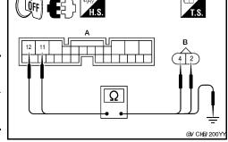
3. Check continuity between differential lock control unit harness connector M70 (A) terminals 11, 12 and ground.
