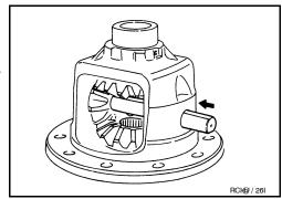
6. Drive a new lock pin into pinion mate shaft, using Tool.
