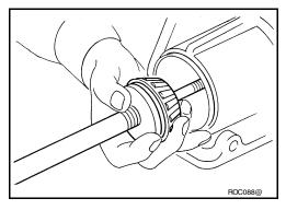
5. Turn the assembly several times to seat the drive pinon bearings.
